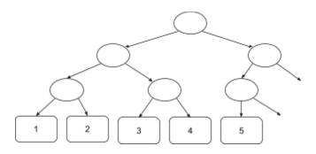
The Merkle tree is grown from the left to the right. Then, once the tree is complete, an extra level is added at the top, and the process is repeated. The original implementation exhibits a peculiar design flaw as empty branches and empty leaves, always positioned to the right by
